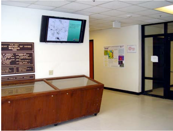
Fig. 1: 42-in plasma display in LME entry from quad. Large cabinet to be removed, allowing installation of kiosk controls. Computer and DVD player driving display are in LME 320 behind wall.
