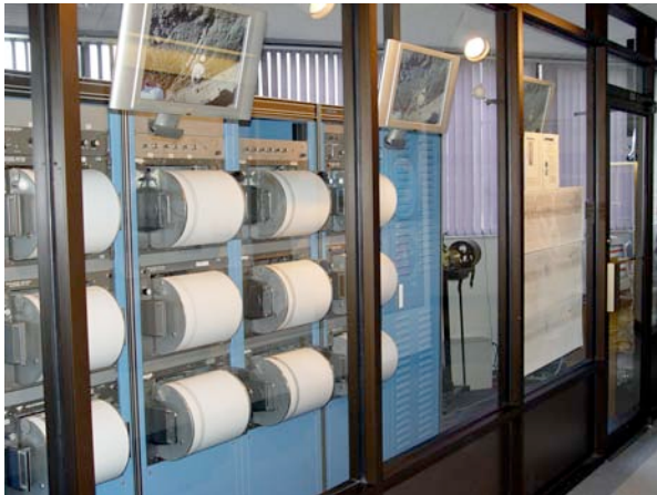
Fig. 3: Three of the four displays, complementing active helicorder drums and static displays on opposite wall.
