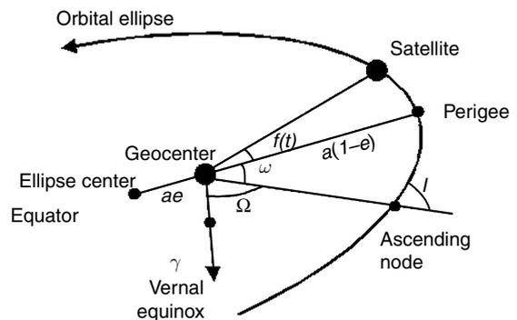
**Figure 5** Diagram illustrating the Keplerian orbital elements: semimajor axis  $a$ , eccentricity  $e$ , inclination  $i$ , argument of perigee (closest approach)  $\omega$ , Right Ascension of the ascending node  $\Omega$ , and true anomaly  $f$  as a function of time  $t$ . The geocenter is the Earth center of mass; hence, satellite geodesy can realize the physical origin of the terrestrial reference system. This diagram is exaggerated, as GPS orbits are almost circular.
