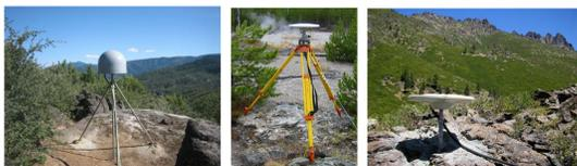
GPS stations: Continuous station (above left), Campaign station (above center) and UNR "MAGNET" station (above right).
